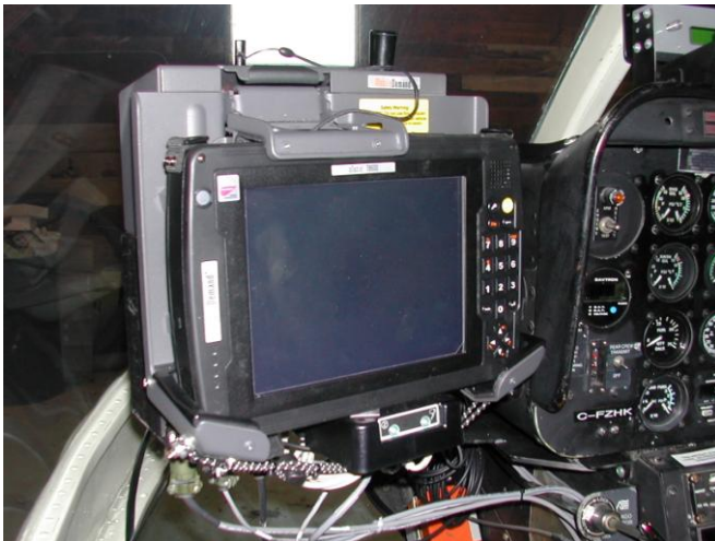
Figure 4: AGIS installed in the Bell 206.
